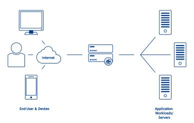
Load balancers are used to provide availability and scalability to the application. The applicati beyond the capacity of a single server. The lo questions that I can help you with? balancer works to steer the traffic to a pool c. available servers through various load balancing
